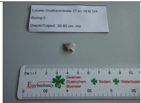
Boring 2 (30-80 cm -mv (Bwp-horizont))
