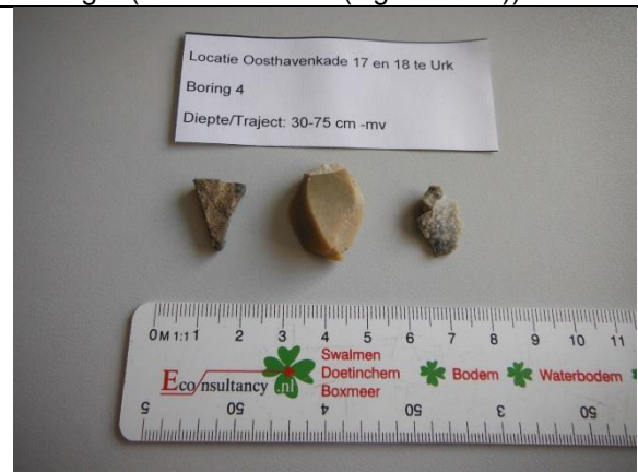
Boring 4 (30-75 cm -mv (Bwp-horizont, geroerde verstoorde laag))
